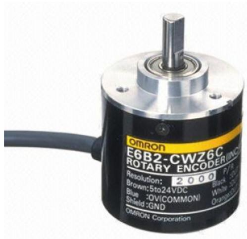
Figura 10 – Encoder incremental Omron - tomado de <https://goo.gl/7Cn4A4>
