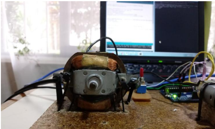
Figura 66. Control On/Off carga AC
