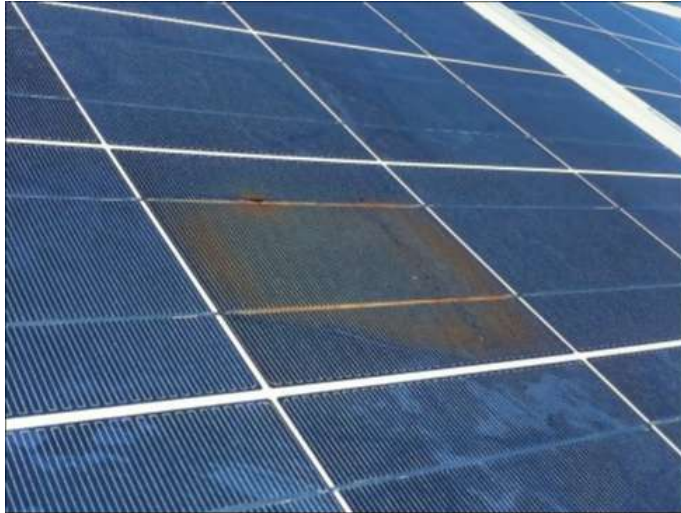
Figure 1.3: EVA degradation in PV panel. Adapted from: [14]
