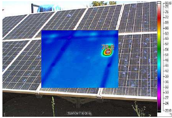
Figure 1.9: PV panel with hot spot. Adapted from: [33]
