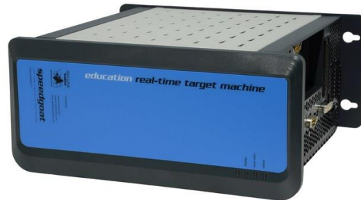
Figura 4. “Speedgoat” Education Real-Time Target Machine (Promod, s.f)
