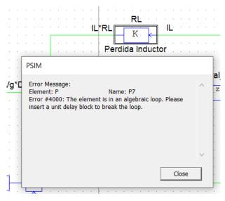
Figura 27. Error #4000 unit delay
