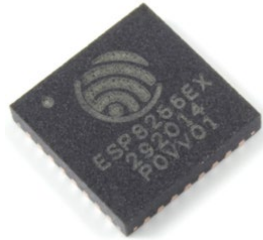
Figura 5: Wifi chip ESP8266EX
