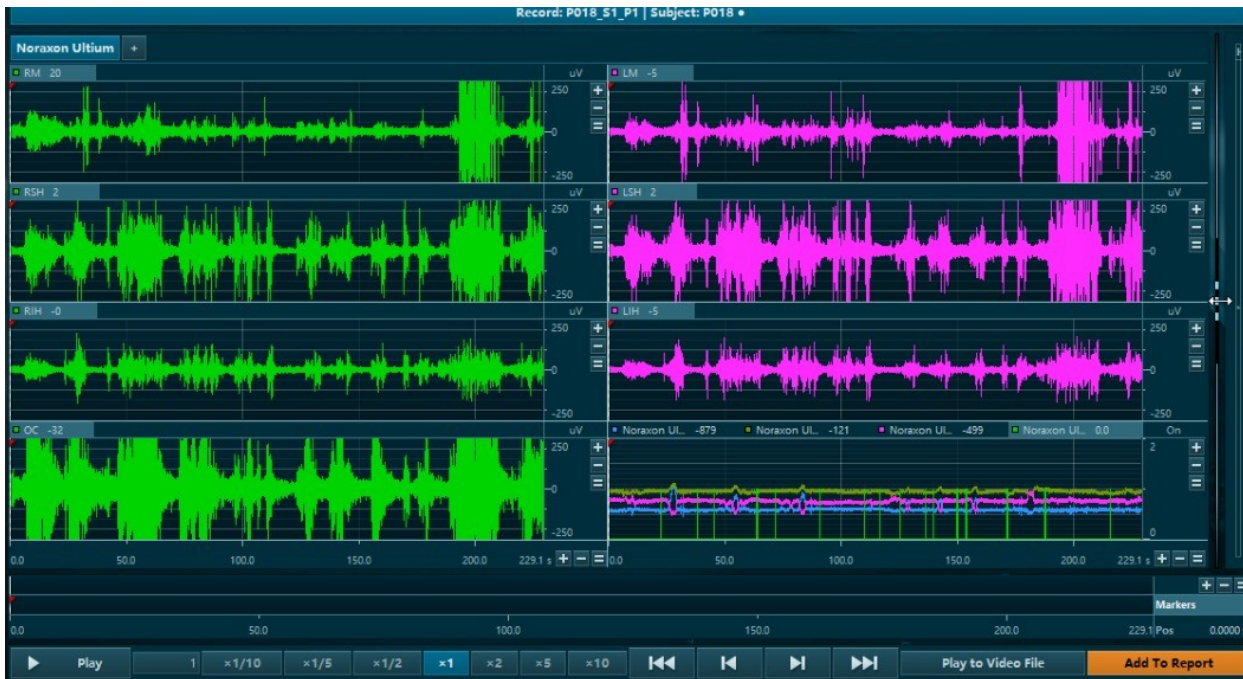
Figure 2-2.: Seven sEMG channels visualization in the MR3 software (Noraxon USA) during the swallowing of 10 mL yogurt bolus. RM and LM, right and left masseters; OC indicates orbicularis oris ; RSH and LSH, right and left suprahyoid muscles; RIH and LIH, right and left infrahyoid muscles. The three signals showed at the bottom right of the figure are 3-axis accelerometry signals, which were not analyzed in the present master's thesis.
