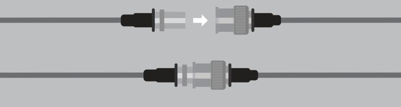
If you need to water proof a BNC connection, we highly recommend using a product like *Coax-Seal* to safely cover and prevent any water damage that may occur.
