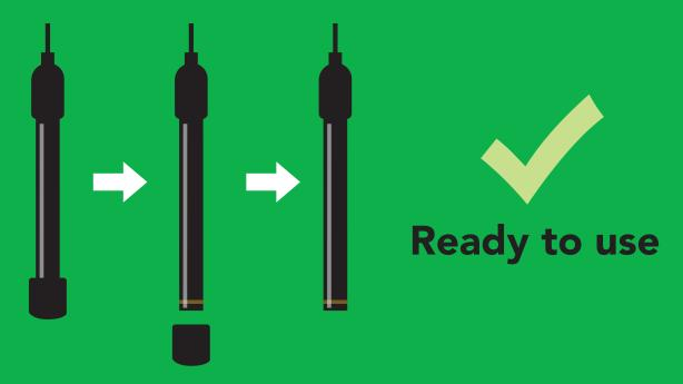
Be sure to watch out for air bubbles, as they can get caught between the two graphite plates and throw off your results. Lightly tap your conductivity probe to knock out any bubbles caught in the probe.
