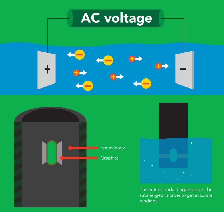
A conductivity probe is a very simple device. It is just two conductors with a fixed surface area at a fixed distance from each other. This distance and surface area is known as the conductivity cell. The cells distance and surface area is quantified as the conductivity cells K constant.
