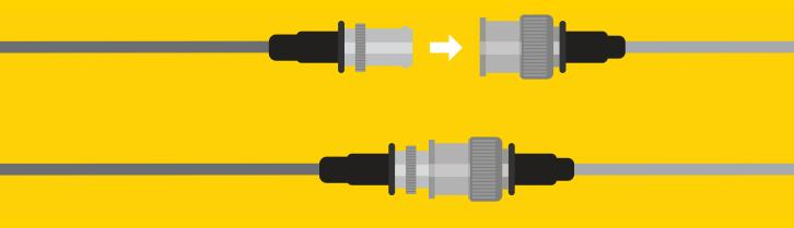
If you need to water proof a BNC connection, we highly recommend using a product like **Coax-Seal** to safely cover and prevent any water damage that may occur.
