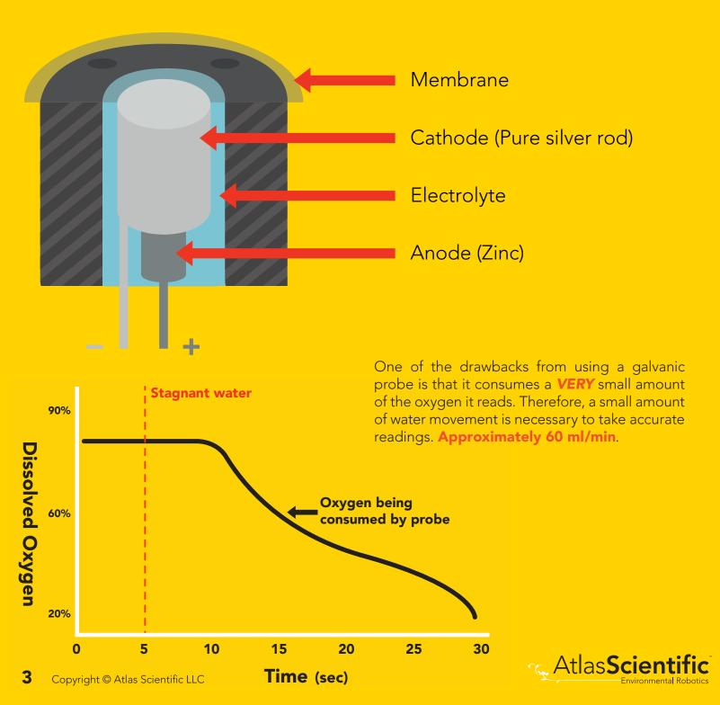
This galvanic dissolved oxygen probe is a passive device that generates a small voltage from 0mv - 40 + mv depending on the oxygen saturation of the Teflon sensing membrane. This voltage can easily be read by a multimeter or an analog to digital converter.
