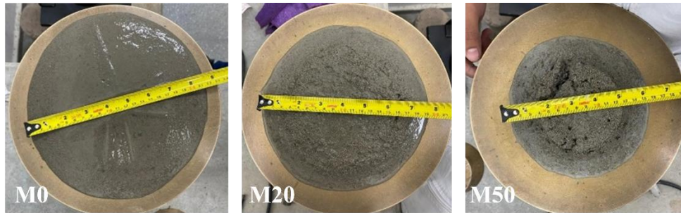
Figure 5. Flow decreases as GPW increases. The photographs show the changes in workability for mixtures M0, M20, and M50. Source: own elaboration.
