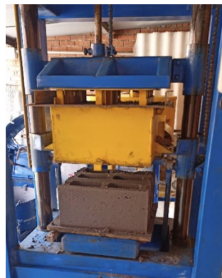
Figure 7. Blocks released from the vibro-compactor. Source: own work.
