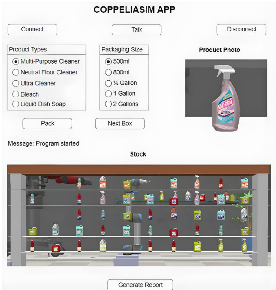
Figure 9. Simulation of the packaging and inventory distribution process in CoppeliaSim. Source: own elaboration.
