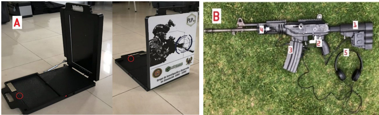
Figure 1. System parts. A) Views from the target of the Portable Laser Polygon, a red circle indicates the camera location used to capture images during a shooting practice. B) Elements arranged to the Galil ACE 23 rifle, (1) electromechanical recoil system, (2) trigger, (3) power supplier, (4) laser coupling, (5) headphones to provide auditory immersion during a shooting practice. Source: own elaboration.
