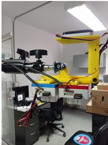
Figure 3-13: PLA-designed to integrate the tripod and cameras.
