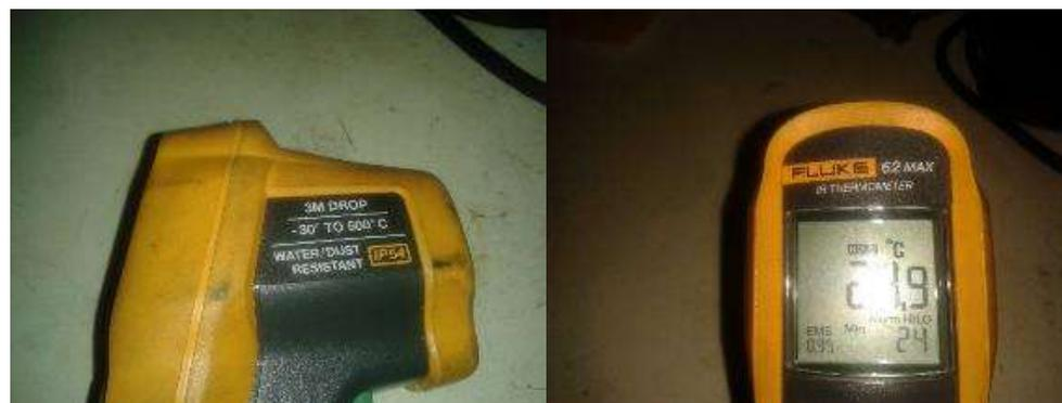
**Figura 29.** Sensor infrarrojo de temperatura Fluke 62 Max ([www.fluke.com/fluke/coes/Termometros/](http://www.fluke.com/fluke/coes/Termometros/))
