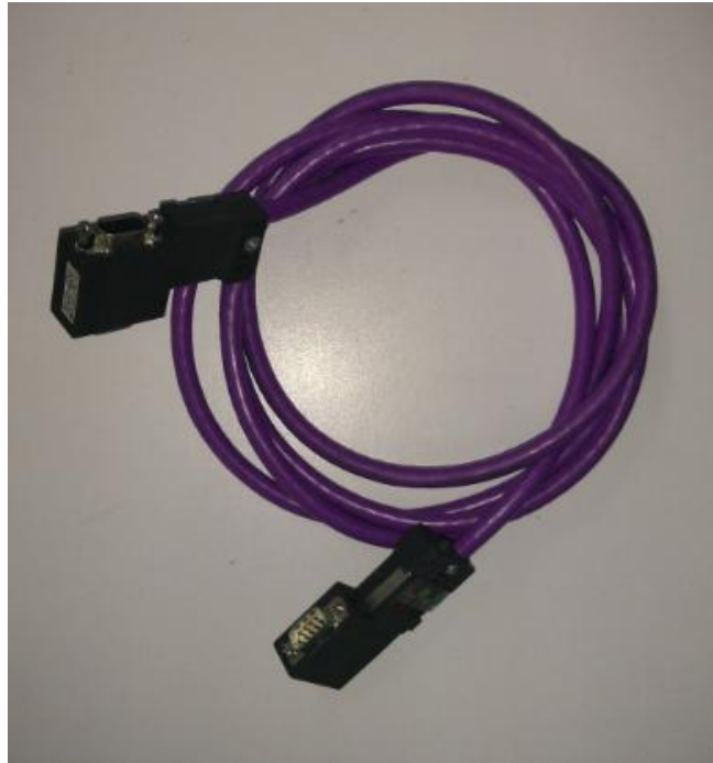
Figura 61. Cable Profibus DP.
