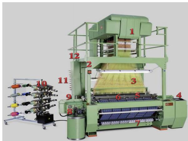
**Figura 7 Partes de Telar Muller Mugrip 5**
