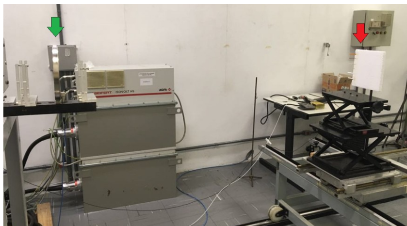
Figure 3 - Setup for irradiation film strips (green and red arrows indicate the position of X-ray tube and film strips).
