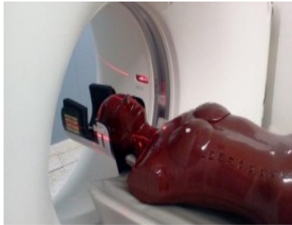
Figure 1.- Alderson Rando phantom positioned in the CT scanner.
