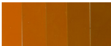
Figure 2 – Intensity color variation degree by irradiation, reference strip and irradiated strips irradiated with increasing doses from the left.
